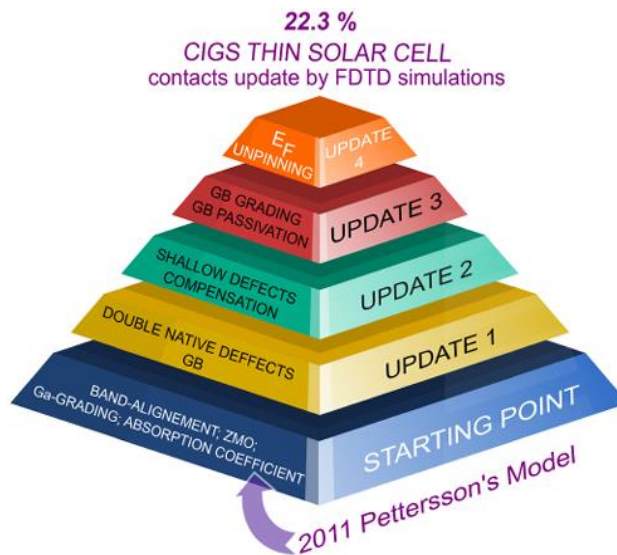
Figure 7 Progressive refinement of the SCAPS-1D baseline model for ultrathin CIGS solar cells (Violas et al. [22]), illustrating successive calibration steps from a basic single-layer absorber to an advanced structure incorporating: (i) a surface defect layer (SDL) at the CdS/CIGS interface, (ii) post-deposition treatment (PDT) effects of alkali fluoride (KF, RbF, CsF) passivation, and (iii) optical boundary conditions from electromagnetic modeling. Each update narrows the gap between simulated and experimentally certified device parameters ( V_{OC} , J_{SC} , FF, PCE), thereby establishing a calibration framework that is transferable to multidimensional TCAD environments. Adapted from Ref. [22].
