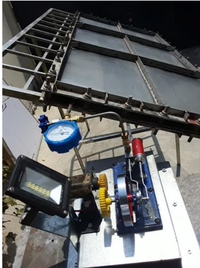
Figure 4 A reciprocally moved steam engine (i.e., a heat engine) along with a pressure gauge, electric generator (DC electricity generating device), and an LED bulb attached to an SLAPE solar panel exposed to natural sunlight [46].
