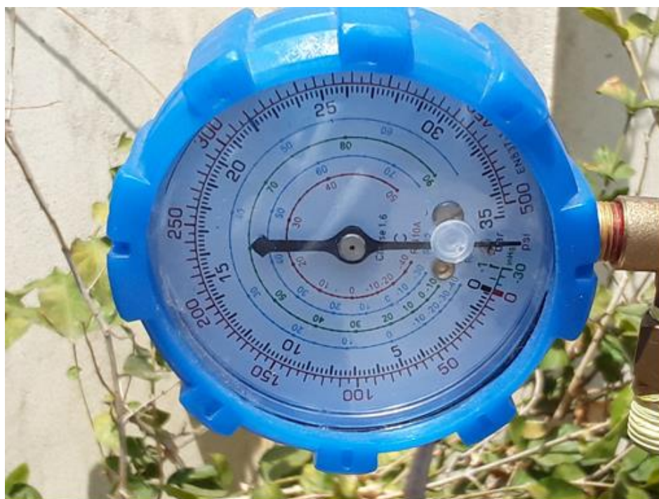
Figure 3 A pressure gauge connected to a manifold of a copper tube conduit attached to the SLAPE solar panel showing in situ generated pressure out of dichloromethane working fluid (WF) upon exposure to the natural sunlight between 9 am and 1 pm on 29 th March 2022 [46].
