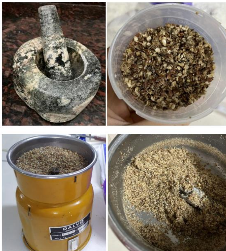
Figure 4 Ground seeds obtained using a stone mortar (top) and a laboratory blade mill (bottom).
