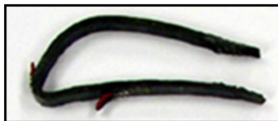
Figure 13 Typical final State of the Failed CMC Vane Specimens [31].
