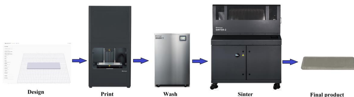
Figure 5 The workflow of the Markforged metal printing process.
