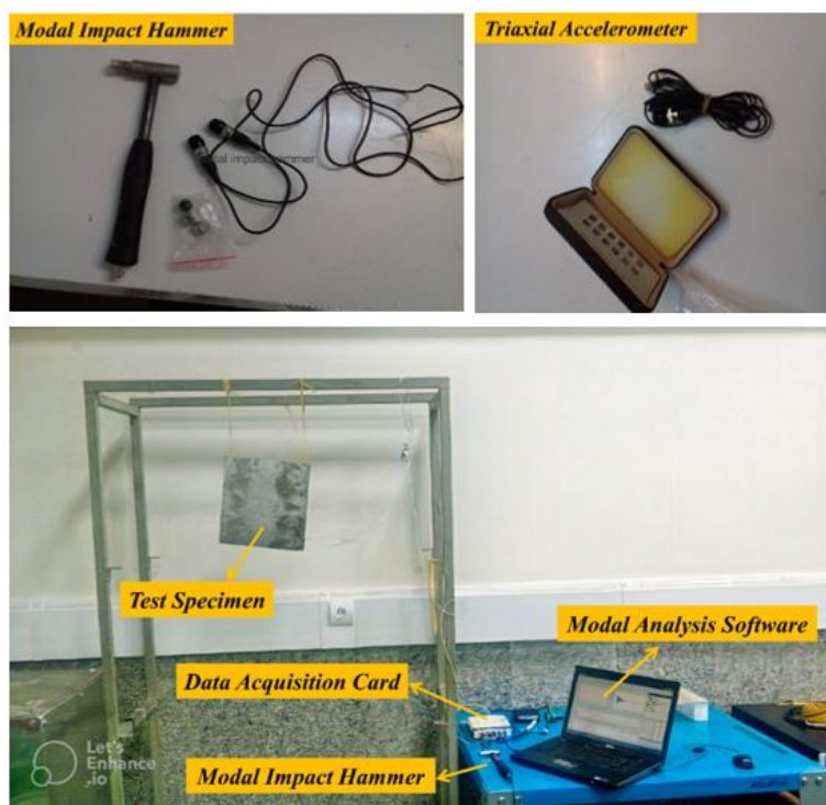
Figure 5 Experimental set-up to conduct modal analysis.
