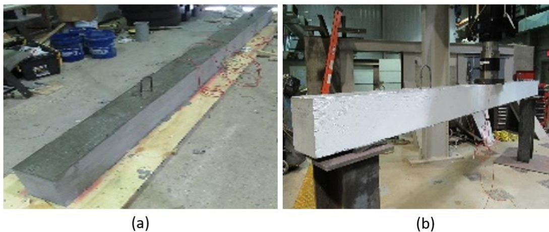
Figure 7 UHPC beam after concrete pour. (a) beam after form removal. (b) beam erected on supports.
