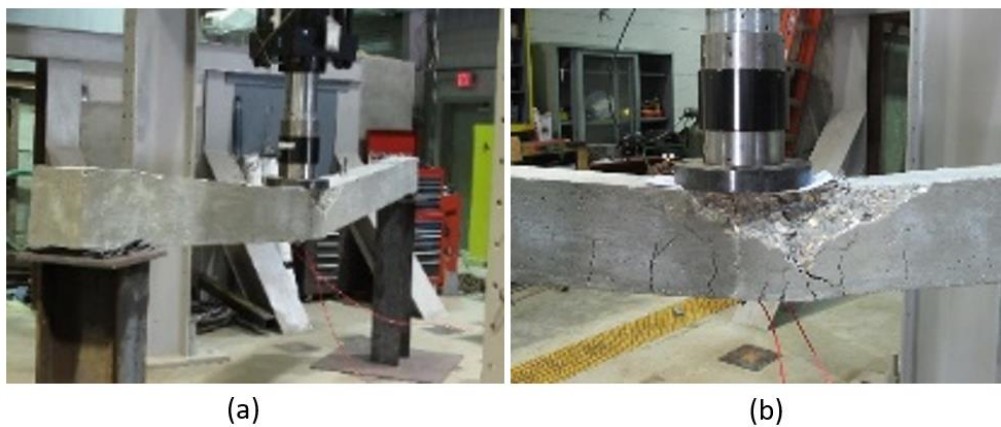
Figure 10 Conventional beam test. (a) beam during testing. (b) beam failure.
