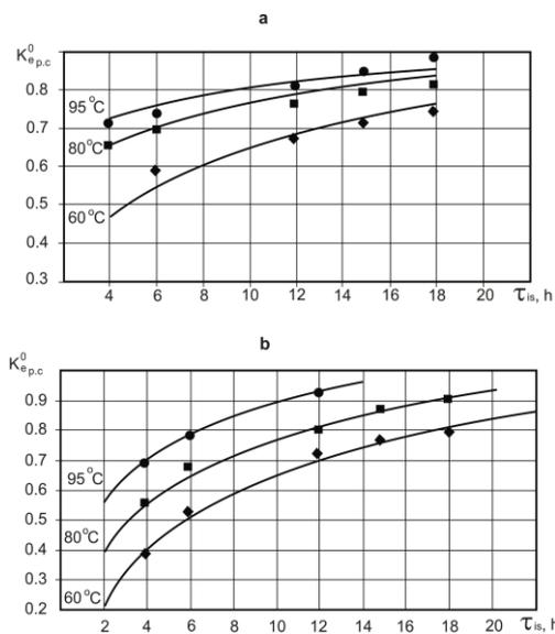
**Figure 1** Graphs for determining coefficients  $K_e^0$ : *a* - using Portland cement; *b* - using Portland Slag cement;  $\diamond$  -  $t_{t,t} = 60^\circ\text{C}$ ;  $\square$  -  $t_{t,t} = 80^\circ\text{C}$ ;  $\circ$  -  $t_{t,t} = 95^\circ\text{C}$ .
