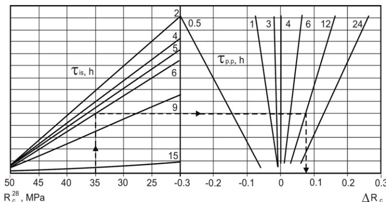
**Figure 2** Nomogram for calculating the increase in relative concrete strength  $\Delta R_c = K_t \lg(\tau_{p,p}/\tau_{p,p}^0)$  after steaming and poststeaming period up to 1 day.
