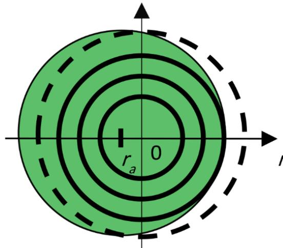
**Figure A1** Field generated by the magnet when the axis of the superconductor is at position  $r_a$  with respect to the magnet axis. The full lines show points of the superconductor threaded by the same field magnitude located along circles, while the dash line shows points of the superconductor threaded by the same field magnitude that are located along an arc of a circle.
