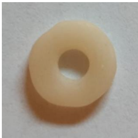
Figure 2 A feldspathic ceramic test specimen with a rough surface.
