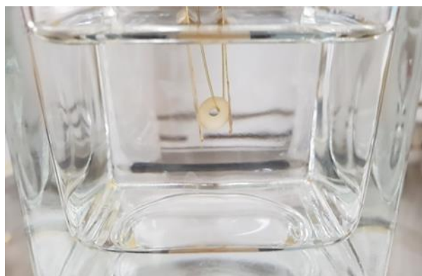
Figure 4 A zirconium dioxide ceramic test specimen with double-sided contact with the gold sheet electrodes in the electrolyte.
