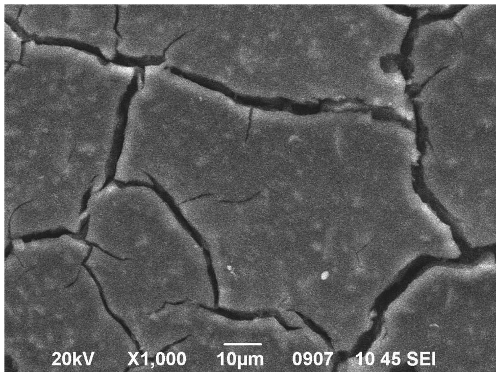
**Figure 1** Representative scanning electron microscopy (SEM) image of the surface of a high-viscosity glass ionomer cement Equia Fill after desiccation presents microcracks.
