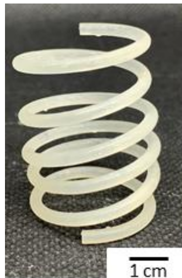
Figure 1 3D printed parts used on the work for investigating the copper electroplating process. The as-printed shape memory polymer (left), the conductive coating applied only to a spiral pattern on the part (middle), and the copper traces after electroplating the ink (right).
