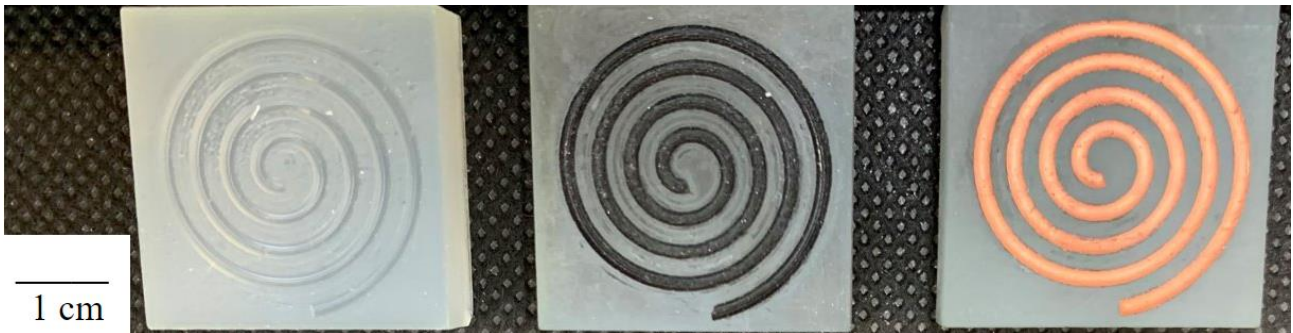
Figure 1 3D printed parts used on the work for investigating the copper electroplating process. The as-printed shape memory polymer (left), the conductive coating applied only to a spiral pattern on the part (middle), and the copper traces after electroplating the ink (right).
