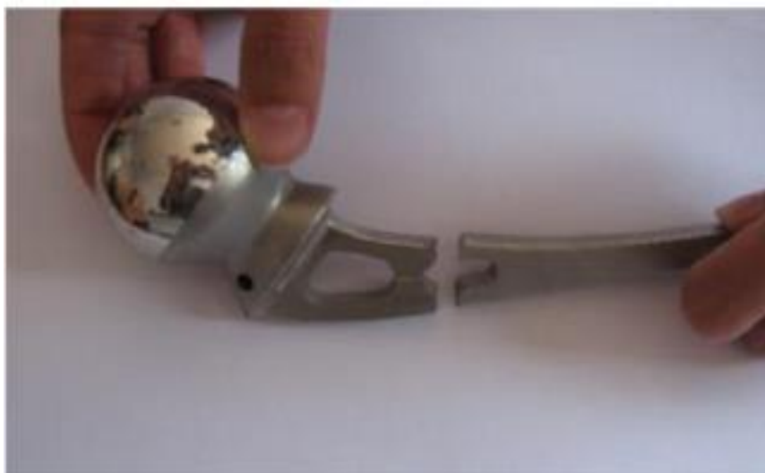
Figure 7 Failure of an artificial hip prosthesis [53].
