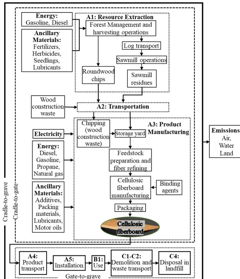
Figure 1 Cradle-to-grave system boundary for CFB manufacturing system.
