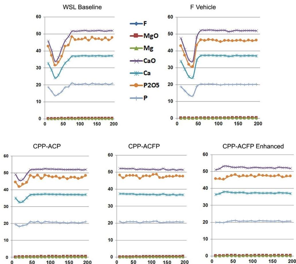
**Figure 9** EPMA results arranged according to the treatment group, showing proportions in weight percent on the vertical scale, versus distance from the enamel surface on the horizontal scale. Data show mean values for N = 15 points at each sample location. The initial WSL at baseline had a depth of ~100 μm. Treatment with CPP-ACFP restores the profile of the treated area to that of normal enamel.
