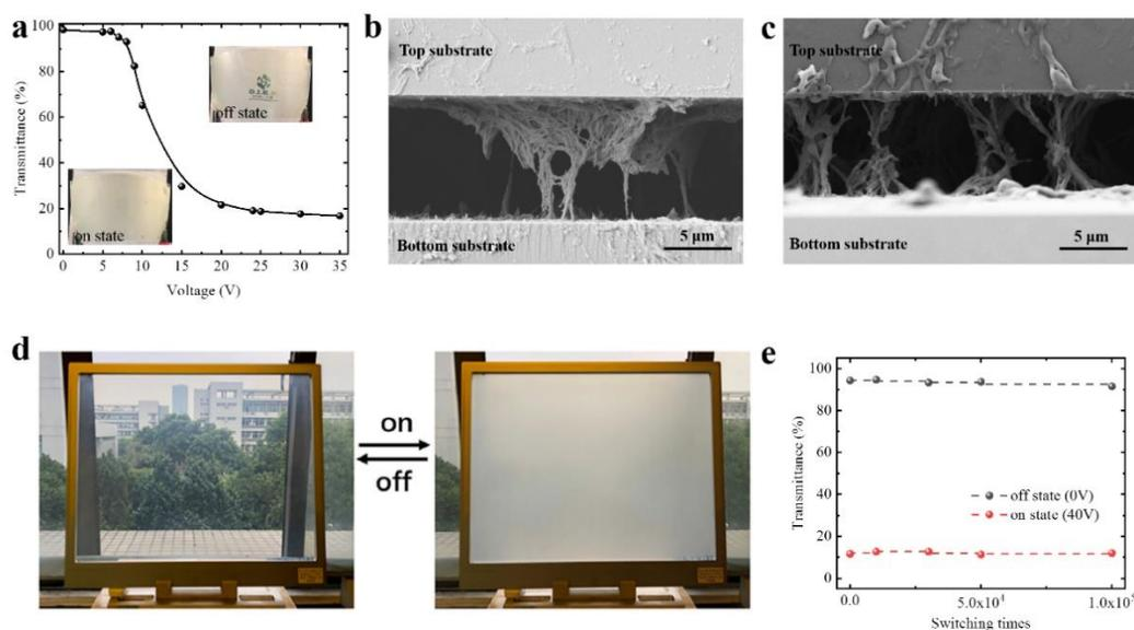
**Figure 4** a) Electro-optical performance and images of PSLC fabricated on the flexible substrate in the OFF/ON states [34]. Cross-sectional SEM images of the polymer networks (for PSLC) with alignment layers fabricated using b) polyimide and c) bi-functional silanes [35]. d) Prototype of a G2.5 size PSLC smart window in the OFF/ON state [28]. e) Transmittance recorded for a PSLC in the OFF and ON states as a function of switching times [28].
