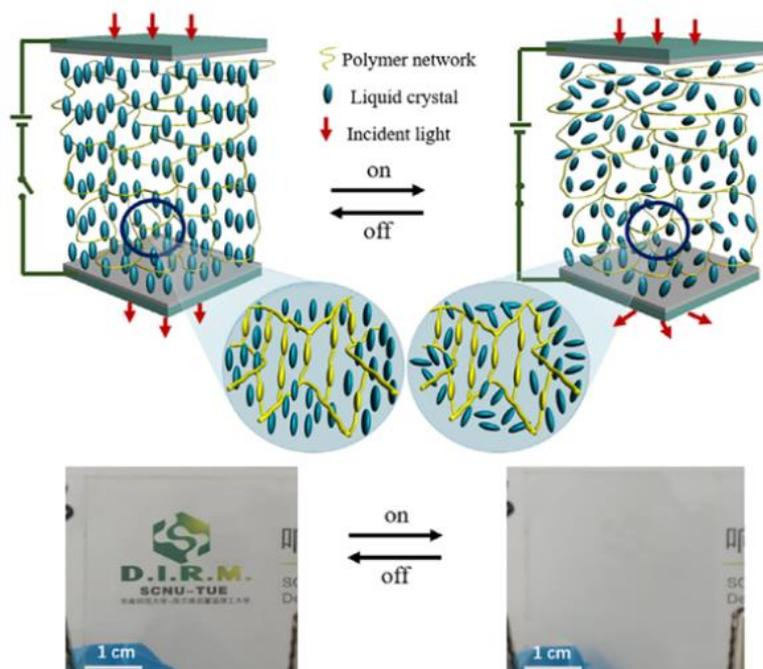
**Figure 2** Schematic representation of the working principle and images of PSLCs in their OFF/ON states [28].
