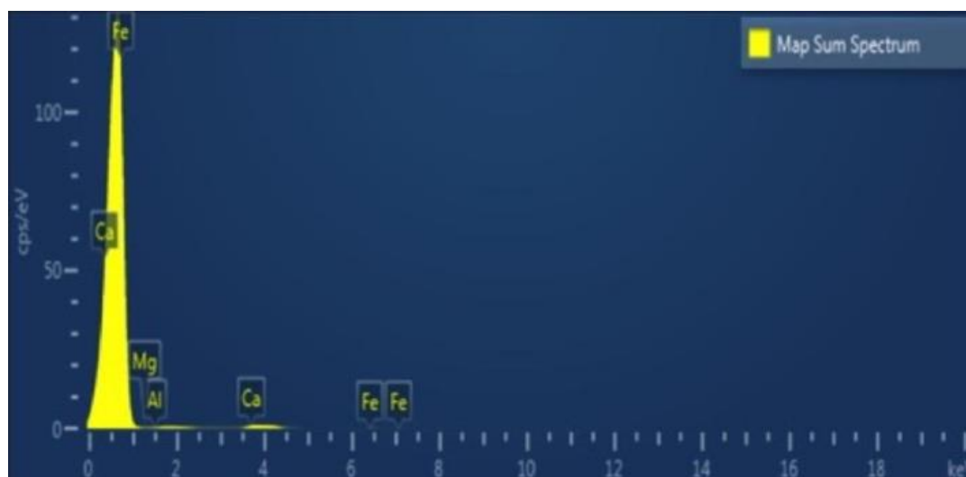
Figure 4 Energy dispersive X-ray (EDX) measurement of the large particle in the highlighted region of the SEM image (Figure 3b) of sample A.
