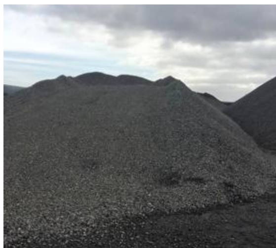
Figure 1 Photographs of basic oxygen steelmaking (BOS) slag pile from which sample A was collected at Tata Steel, Port Talbot on 20 th October 2017.
