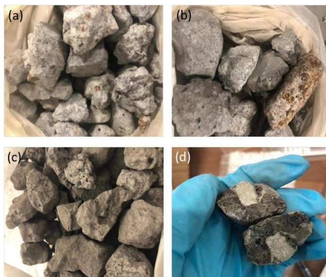
Figure 2 Photographs of basic oxygen steelmaking (BOS) slag samples: (a) sample A, (b) sample B (c) sample C, and (d) a piece of sample A slag illustrating the presence of a free lime pocket. All sample were obtained from Tata Steel, Port Talbot on 20 th October 2017.
