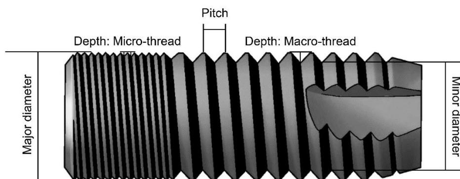
**Figure 3** The definitions of thread depth and pitch. Notably, the difference between micro and macro-threads is thread depth. This figure also shows the major and minor diameters of a screw. It is notable that, in implantology, the implant diameter means the major diameter.
