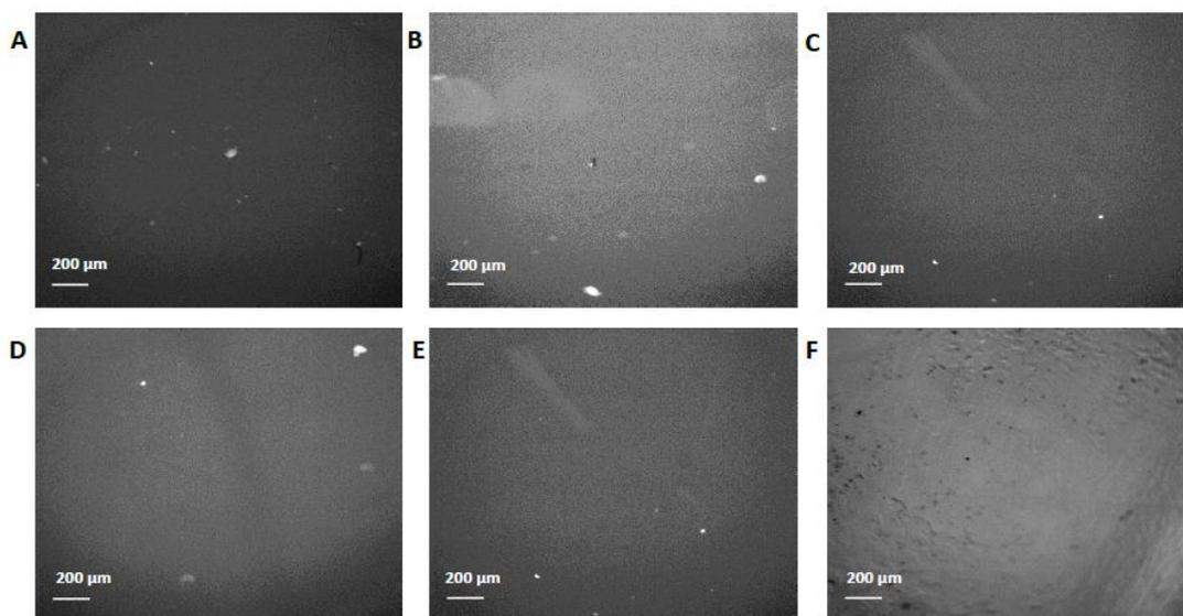
**Figure 3** Representative fluorescent images of different surfaces (4× magnification) prior to blood contact. Top (bare surfaces): A) PC, B) PVC, and C) PS; bottom (MEG-OH-coated surfaces): D) PC, E) PVC, and F) PS. Dark areas represent defect- or contamination-free surfaces.
