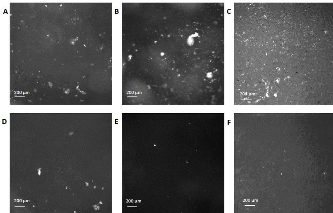
**Figure 5** Representative fluorescent images of different surfaces (4× magnification) after 6 hours of blood contact. Top (bare surfaces): A) PC, B) PVC, and C) PS; bottom (MEG-OH-coated surfaces): D) PC, E) PVC, and F) PS. Dark areas represent (platelet-free) polymer surfaces (bare or MEG-OH-derivatized) and the bright areas represent attached fluorescently-labelled platelets.
