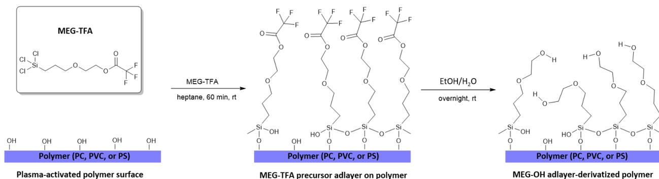
**Figure 1** Schematic representation of the straightforward, two-step surface modification of polymer (PC, PVC, or PS) surface with antithrombogenic MEG-OH surface chemistry.
