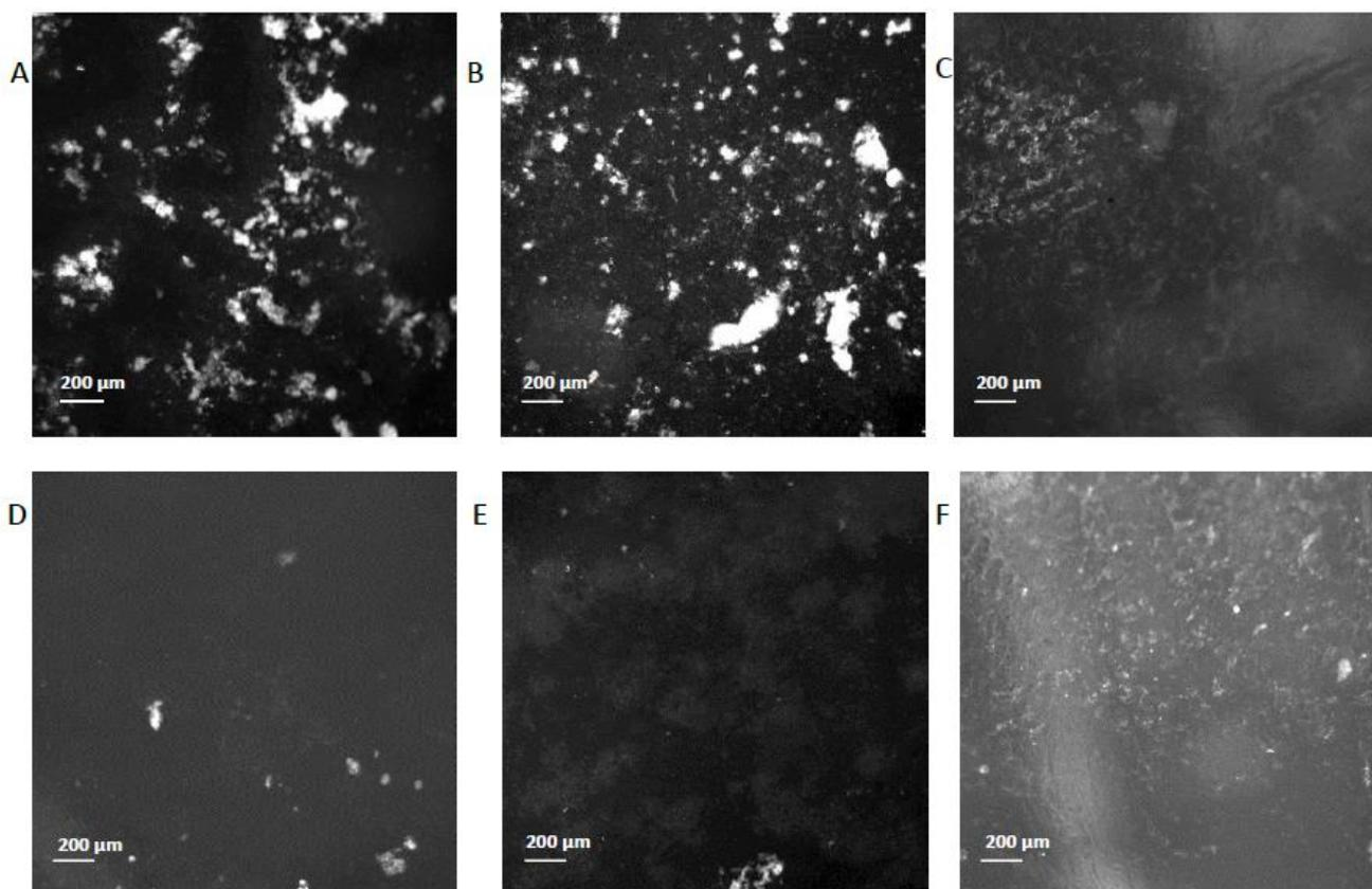
**Figure 4** Representative fluorescent images of different surfaces (4 $\times$  magnification) after 3 hours of blood contact. Top (bare surfaces): A) PC, B) PVC, and C) PS; bottom (MEG-OH-coated surfaces): D) PC, E) PVC, and F) PS. Dark areas represent (platelet-free) polymer surfaces (bare or MEG-OH-derivatized), and the bright areas represent attached fluorescently-labelled platelets.
