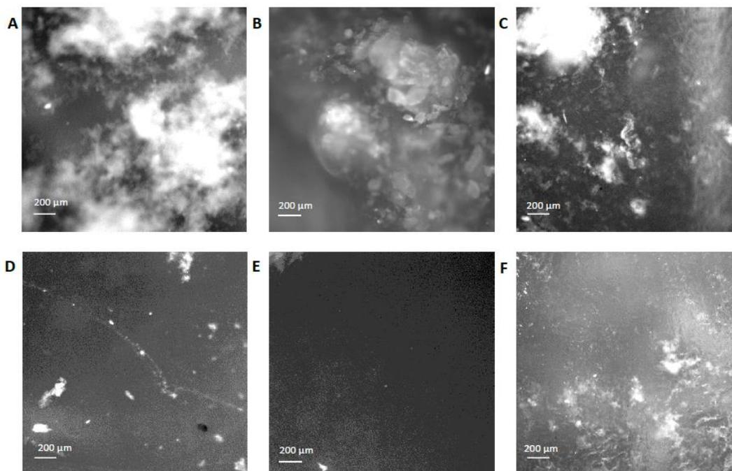
**Figure 6** Representative fluorescent images of different surfaces (4× magnification) after 3 days of blood contact. Top (bare surfaces): A) PC, B) PVC, and C) PS; bottom (MEG-OH-coated surfaces): D) PC, E) PVC, and F) PS. Dark areas represent (platelet-free) polymer surfaces (bare or MEG-OH-derivatized) and the bright areas represent attached fluorescently-labelled platelets.
