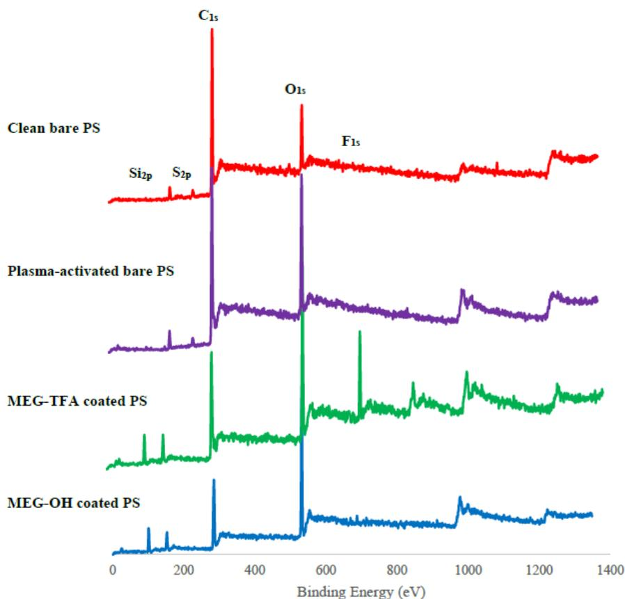
**Figure 2** XPS surveys for (top to bottom) clean bare PS (red), plasma-activated bare PS (purple), as well as MEG-TFA (green) and MEG-OH (blue) coated PS. XPS surveys for bare and MEG-OH-coated PC and PVC are found in references 25 and 26, respectively.
