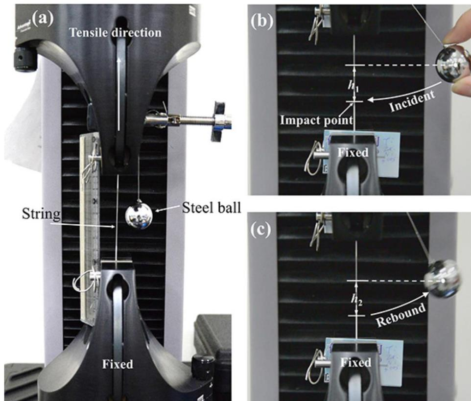
**Figure 2** (a) Setup of the modified ball-drop test, (b) the initial height,  $h_1$ , of the steel ball prior to release, and (c) the captured image depicting the rebound height,  $h_2$ , of the steel ball.
