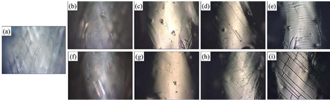
**Figure 5** The optical microscope images of the strings coated with Zr-based and Ti-based TFMGs for different deposition time: (a) Pristine BG65 string without a TFMG coating, (b)-(e) Strings coated with Zr-based TFMGs for 5 min, 30 min, 60 min, and 120 min, respectively, (f)-(i) Strings coated with Ti-based TFMGs for 5 min, 30 min, 60 min, and 120 min, respectively.
