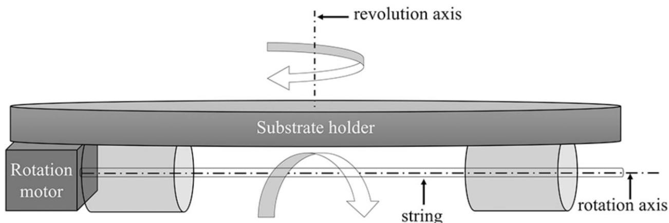
**Figure 1** Schematic drawing illustrating the rotation of the substrate holder with respect to the revolution axis and depicting the home-made string holder for rotating the string with respect to the rotation axis.
