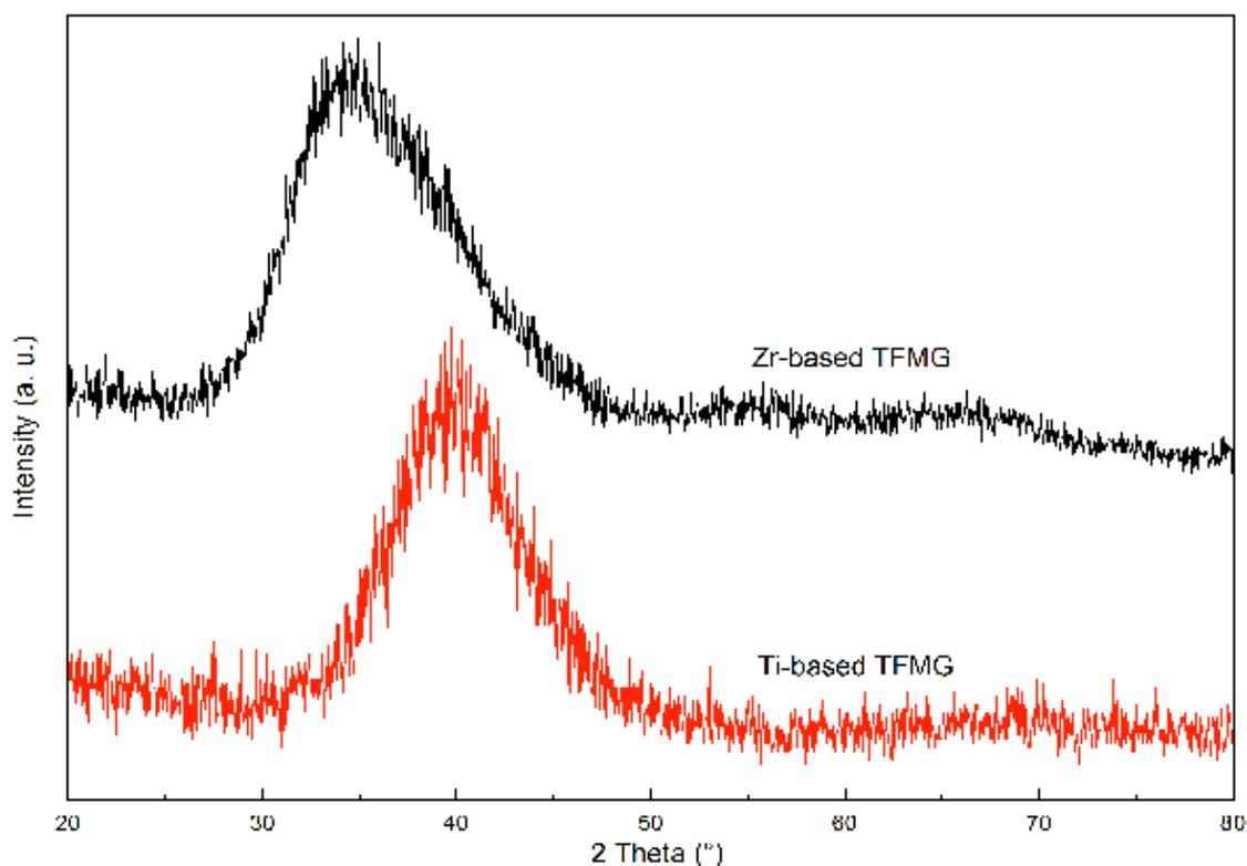
**Figure 3** X-ray diffraction patterns of Zr-based and Ti-based TFMGs.
