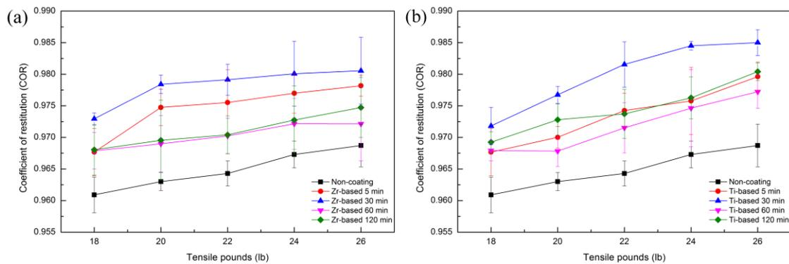
**Figure 7** The COR as a function of tensile loading for (a) Zr-based and (b) Ti-based TFMG coated strings with different coating time.
