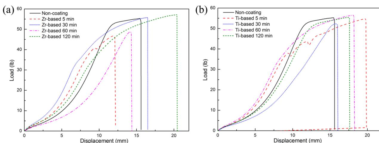
**Figure 8** Tensile load-displacement curves for (a) Zr-based and (b) Ti-based TFMG coated strings with different coating time.
