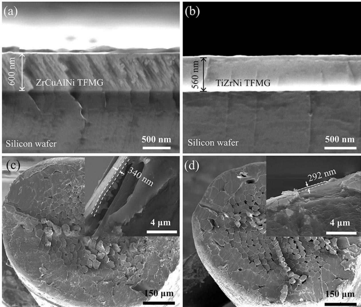
**Figure 4** SEM micrographs showing the cross-sections of (a) Zr-based and (b) Ti-based TFMGs deposited on Si wafer and of (c) Zr-based and (d) Ti-based TFMGs deposited on the rotated string for 120 min, with the inset displaying the coating thickness.
