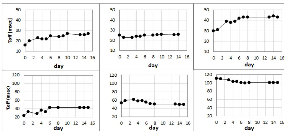
**Figure 8** Time variation of  $\tau_{off}$  in P025-40 (top) & P025-49.5 (bottom) PDLC films at 380 (left), 634 (center) and 1268 (right)  $\text{mJ}/\text{cm}^2$ .
