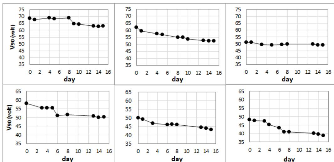
**Figure 6** Time variation of  $V_{90}$  in P025-40 (top) & P025-49.5 (bottom) PDLCs at 380 (left), 634 (center) and 1268 (right)  $\text{mJ}/\text{cm}^2$ .
