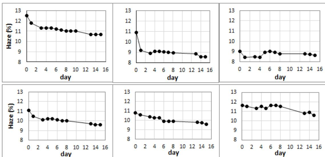
**Figure 2** Time variation of Haze in P025-40 (top) and P025-49.5 (bottom) PDLC films at 38.2 (left), 74.4 and 126.8 (right) mJ/cm<sup>2</sup>.
