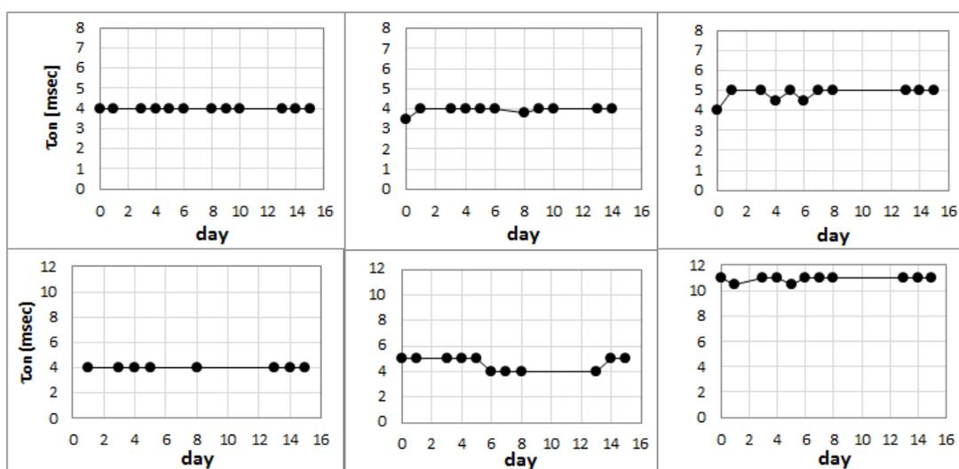
**Figure 7** Time variation of  $\tau_{on}$  in P025-40 (top) & P025-49.5 (bottom) PDLC films at 380 (left), 634 (center) and 1268 (right)  $\text{mJ}/\text{cm}^2$ .
