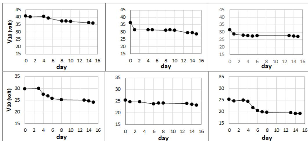
**Figure 5** Time variation of  $V_{10}$  in P025-40 (top) & P025-49.5 (bottom) PDLCs at 380 (left), 634 (center) and 1268 (right)  $\text{mJ}/\text{cm}^2$ .
