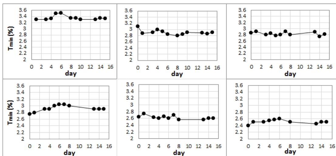
**Figure 4** Time variation of  $T_{min}$  in P025-40 (top) & P025-49.5 (bottom) PDLCs at 380 (left), 634 (center) and 1268 (right)  $mJ/cm^2$ .
