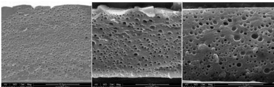
**Figure 1** SEM morphologies of P025-40 films at UV energies of 380 (left), 634 (center) and 1268 (right) mJ/cm<sup>2</sup>.
