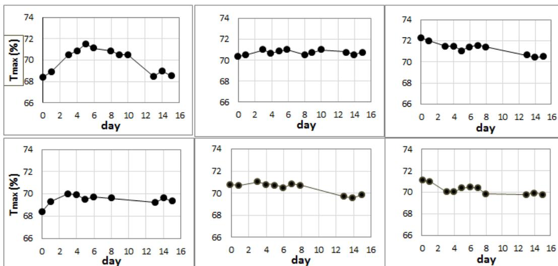
**Figure 3** Time variation of  $T_{max}$  in P025-40 (top) & P025-49.5 (bottom) PDLCs at 380 (left), 634 (center) and 1268 (right)  $mJ/cm^2$ .
