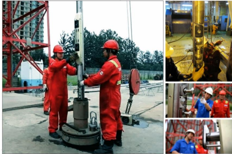
Figure 2 Single and dual probe testers lowered into the well. Courtesy: COSL.
