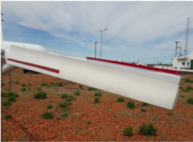
Figure 23 Noise reduction on the SWT, by the modified thickness of the trailing edge.
