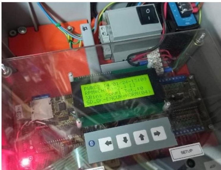
Figure 15 PWRC/2 with recently added AC-coupled power supplies (left), addition of RPM channel with HV input sensor module and (right) regular recalibration of the units.
