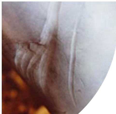
Figure 2 Example of a gouge-dent defect in a tank.
