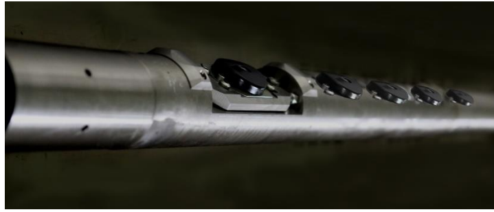
Figure 2 Axial tester - Scanning “array formation tester” concept also provides multiple depths of investigation with different lateral resolutions.
