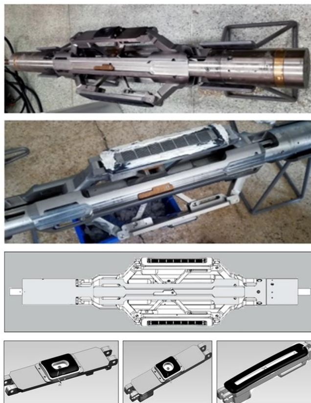
Figure 1 Azimuthal tester – (a) Top two photos, fluid withdrawal from the formation using “small round nozzles” (upper) and “lengthy slotted nozzles” (lower); (b) Middle drawing, long slot nozzles, detailed mechanical assembly; and (c) Bottom drawings, multiple pad varieties support broad pump rate, formation types and permeability/viscosity ranges.
