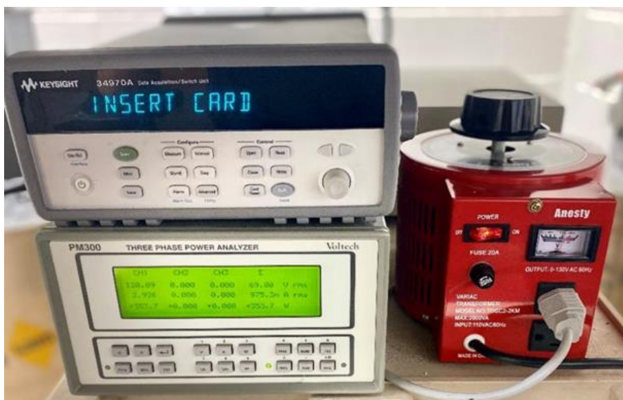
Figure 1 Data Acquisition Device (top left), Power Analyzer (bottom left) and 120 V Power Supply.
