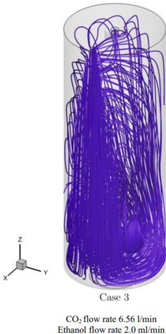
Figure 5 Influence of CO 2 flow rate variations on flow streamlines at a constant flow rate of ethanol.
