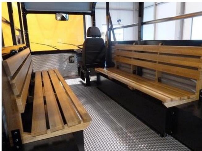
**Figure 4** Wooden facing-type bench.
