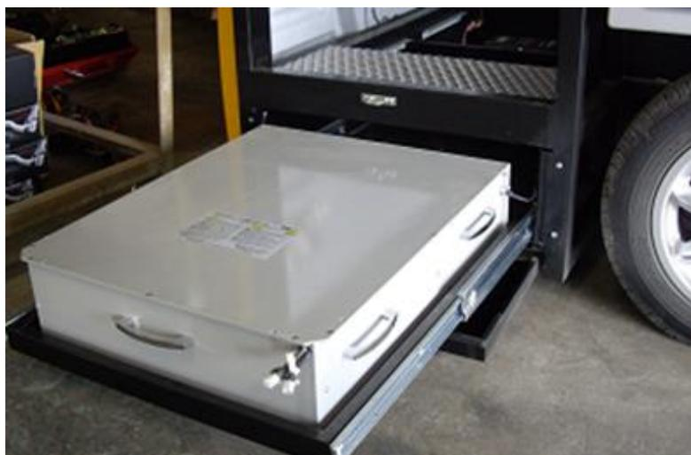
**Figure 5** Exchangeable Li-polymer battery.
