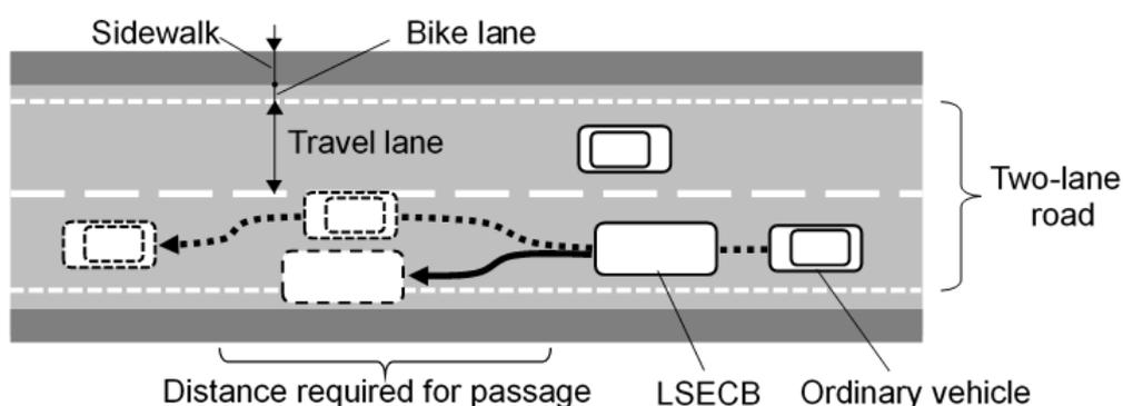
**Figure 8** Typical two-lane road and passing pattern of vehicle.
