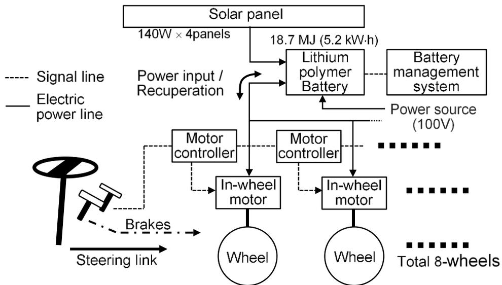
**Figure 6** Block diagram of the power management system.
