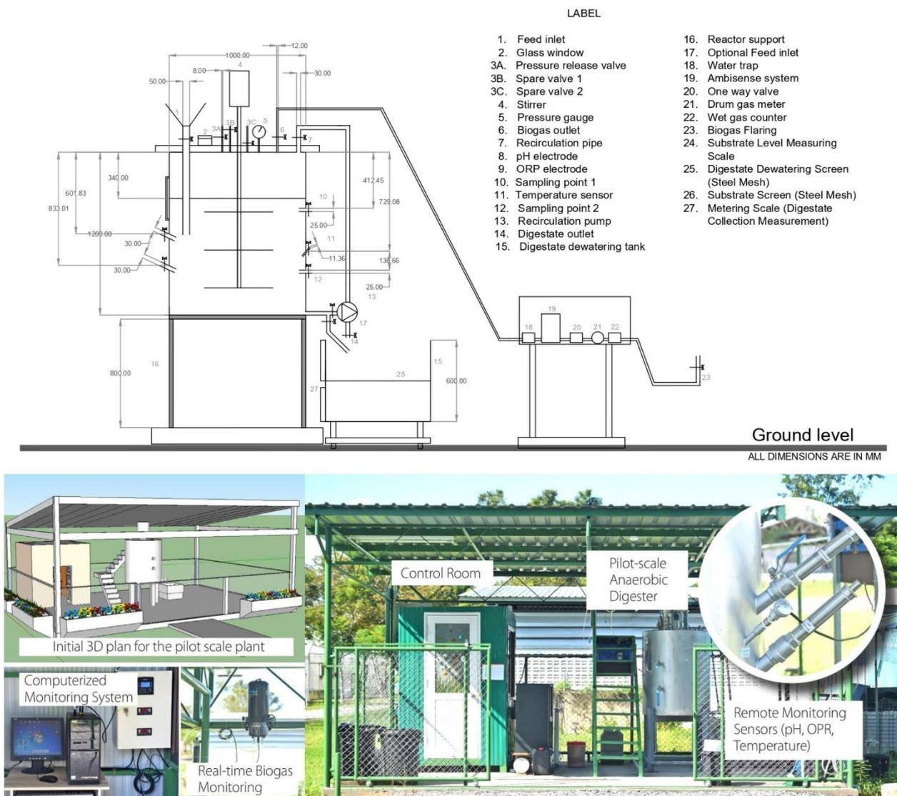
**Figure 2** Top: Schematic of pilot-scale mesophilic anaerobic digester (Thailand); Bottom: Pilot-scale mesophilic anaerobic digester (Thailand).
