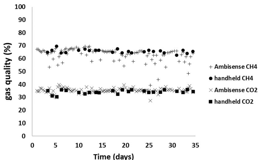
**Figure 5** Comparative gas analyses of CH<sub>4</sub> and CO<sub>2</sub> volumetric concentration from the UK AD unit. GasfluX values are shown with data obtained at the same time using a handheld gas analyser (Gas Data UK – GFM 416).
