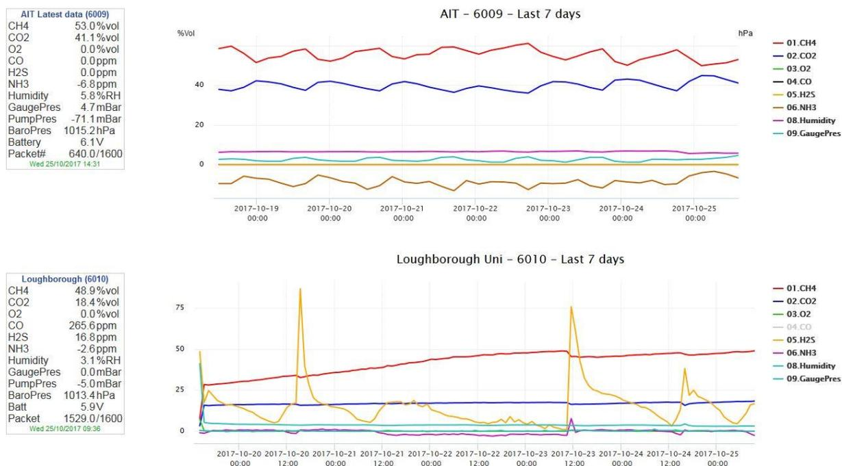
**Figure 3** Screenshot of remotely monitored anaerobic digestion “network” data outputs.
