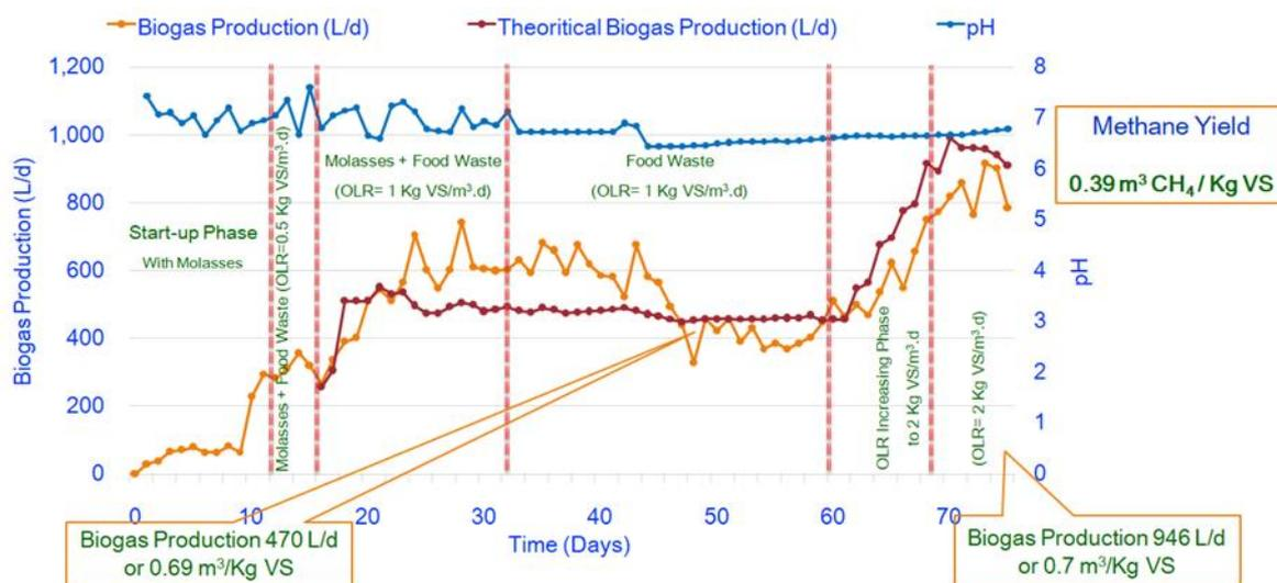
**Figure 4** Daily biogas production and CH<sub>4</sub> Vol.% and pH recorded by the Thailand AD system.
