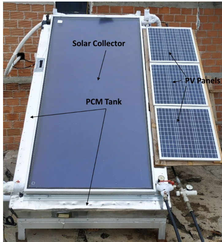
Figure 1 The solar kit unit containing a solar collector, a PCM tank, and PV panels.
