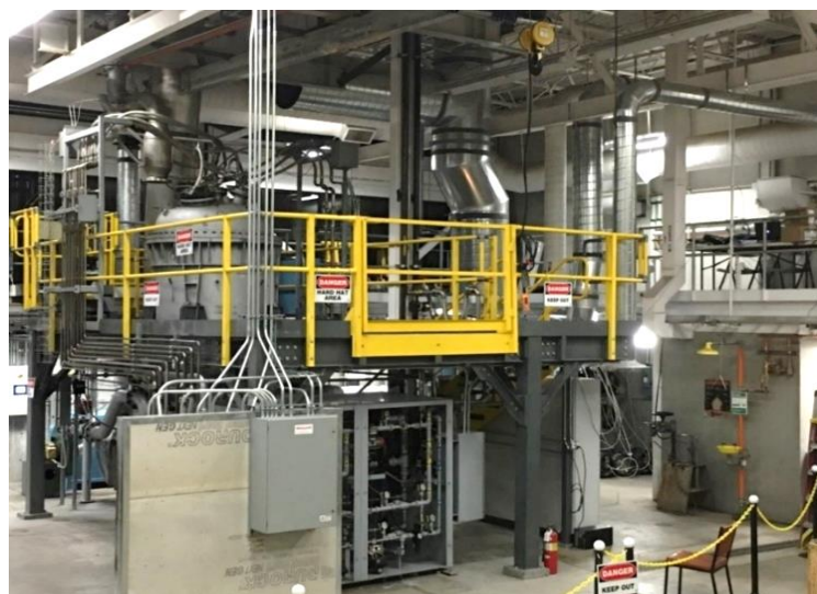
Figure 13 The pilot plant with a flash reactor installed at the University of Utah. [Adapted from M. Elzohiery, Flash Reduction of Magnetite Concentrate Related to a Novel Flash Ironmaking Process, Ph.D. Dissertation, Salt Lake City, Utah: University of Utah, 2018.]
