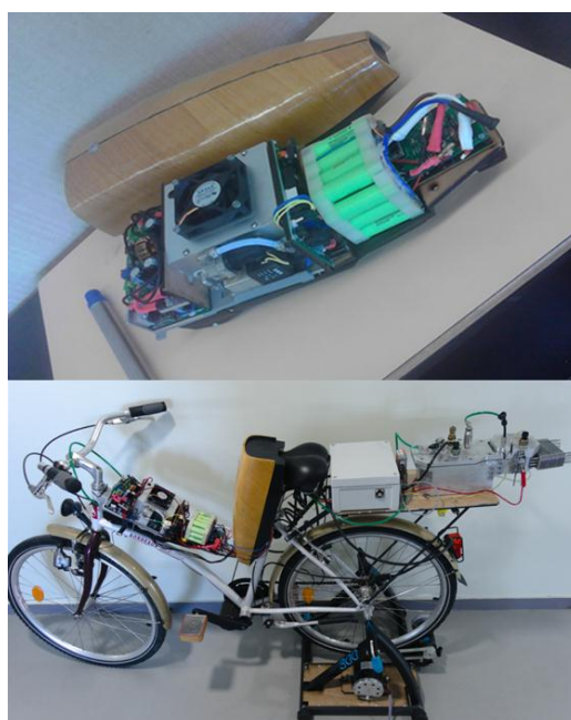
Figure 13 Fuel cell and control kit (up) installed on the bike prototype (down).
