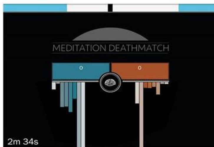
Figure 1 Screenshot of the Meditation Deathmatch User Interface. In this interface, players’ scores are indicated in the blue and orange boxes at the center of the screen. The bars below are moving elements which correspond to proportional levels of each type of brain wave measured by the EEG headset (alpha wave, beta waves, theta waves, etc.). The blue bar at the top of the screen indicates the “meditation value” produced by the Neurosky Mindwave’s internal algorithms and the timer in the bottom of the screen indicates the remaining time left in the round.
