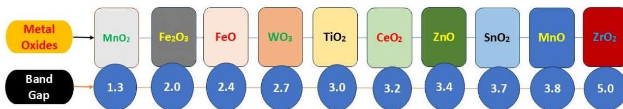
Figure 2 Different band gaps of semiconducting metal oxides [17].
