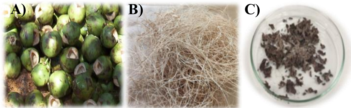
Figure 1 Photographs of (A) discarded coconut, (B) coconut fiber, and (C) ash obtained at a temperature of 800°C.
