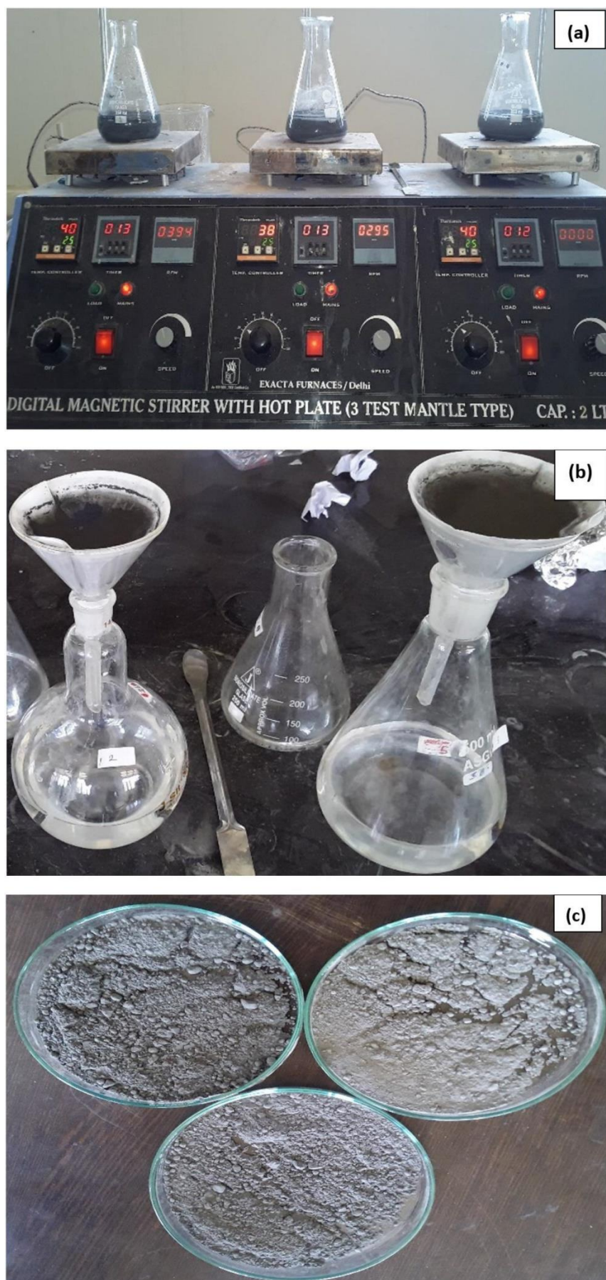
Figure 1 (a) Catalyst Preparation (b) Catalyst Filtration (c) Prepared Catalyst.
