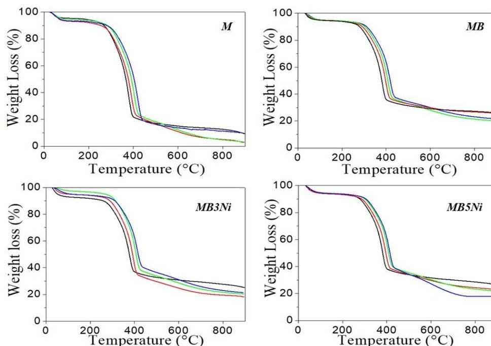
**Figure 1** TG profiles of (a) M, (b) MB, (c) MB3Ni and (d) MB5Ni samples at  $\beta$  heating rates: (•)5, (◻)10, (◻)15 e (◻) 20°C min<sup>-1</sup>.
