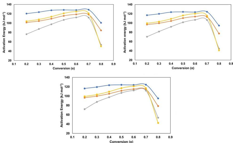
**Figure 3** Activation energy change versus conversion rate for (-) M, (-) MB, (-) MB3Ni and (-) MB5Ni samples.
