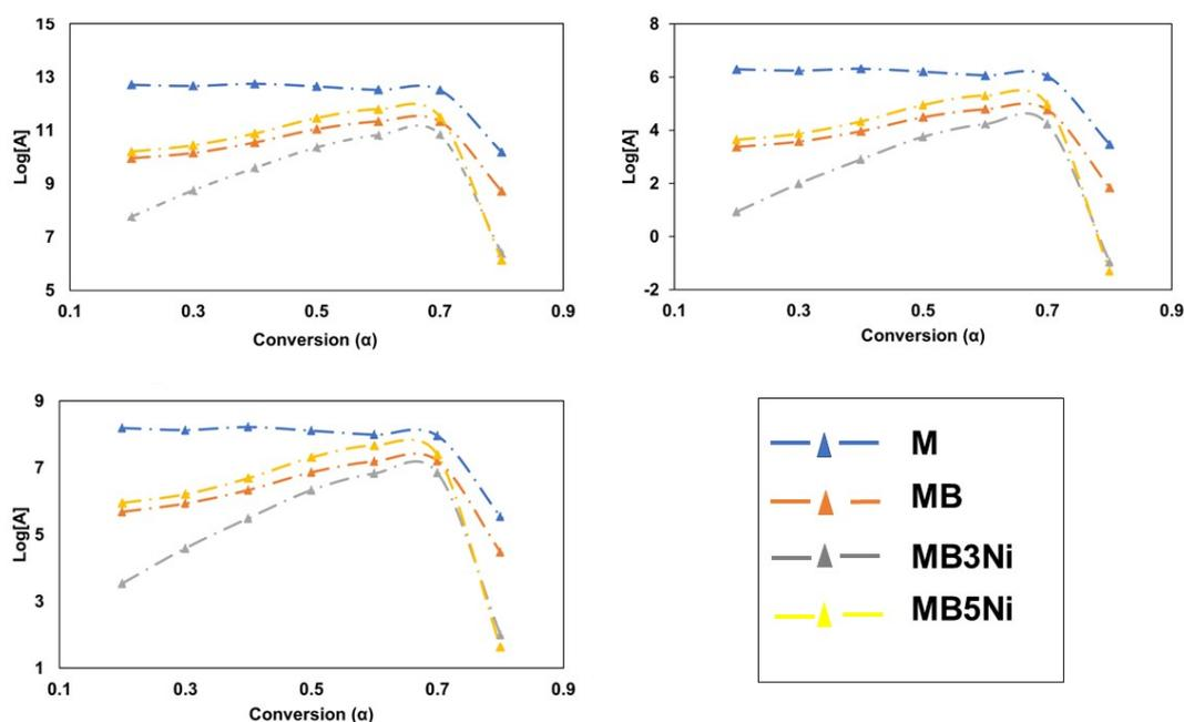
**Figure 4**  $\text{Log}_{10}(A)$  versus conversion ( $\alpha$ ) for catalytic and non-catalytic pyrolysis using FWO, KAS and Friedman models.
