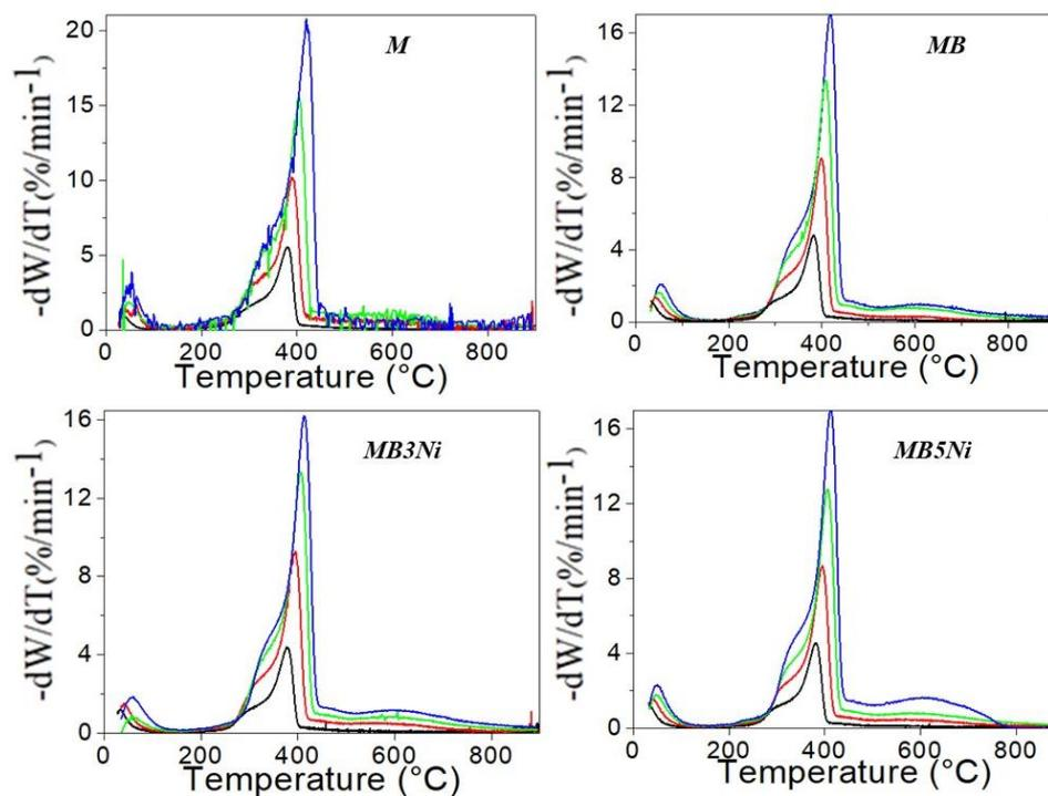
**Figure 2** DTG profiles of samples (a) M, (b) MB, (c) MB3Ni and (d) MB5Ni at heating rates  $\beta$ : (-)5, (-)10, (-)15 e (-) 20°C min<sup>-1</sup>.
