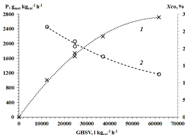
**Figure 2** Dependence of the productivity of the catalyst (1) and the conversion of CO (2) during the synthesis of methanol on the space velocity.
