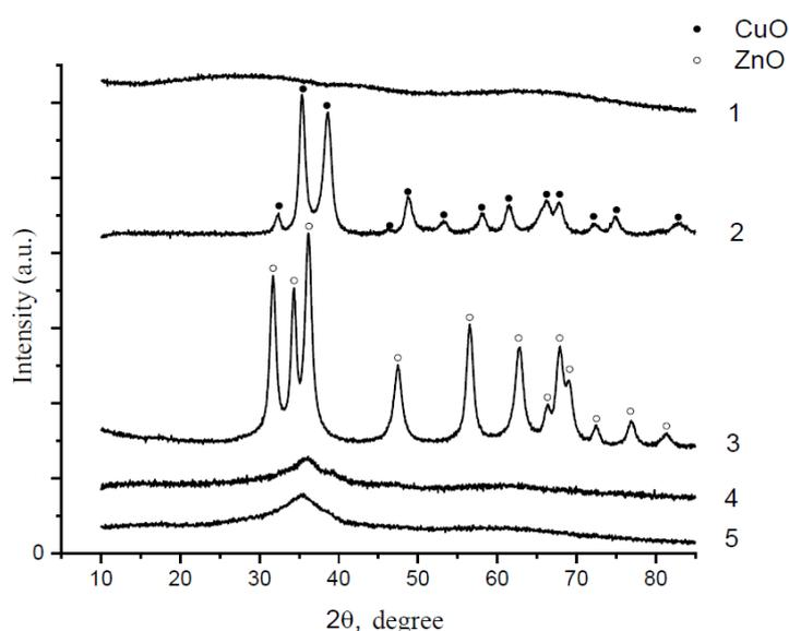
**Figure 1** Diffraction patterns recorded for the samples prepared following the reverse precipitation method (calcination at 300 °C). 1 – Al, 2 – Cu, 3 – Zn, 4 – Cu/Zn/Al, 5 – Cu/Zn.
