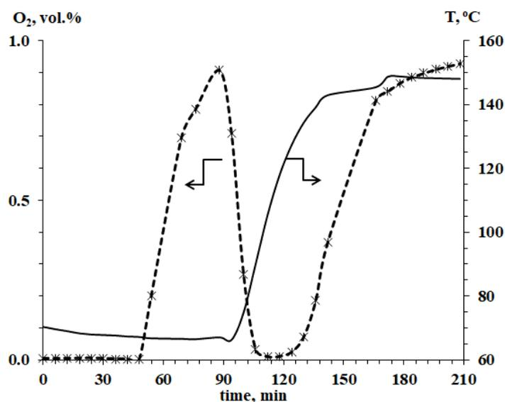
**Figure 4** Dynamics of the oxygen content at the outlet during the oxidation of the catalyst subjected to sintering conditions at 334°C.
