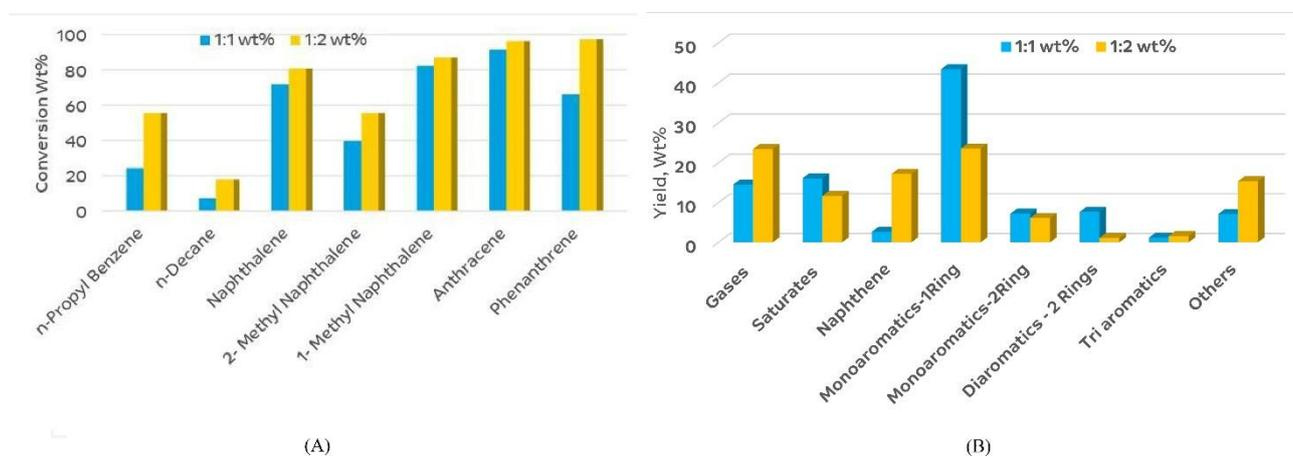
**Figure 6** Effect of Pt/Al<sub>2</sub>O<sub>3</sub> and Y zeolite wt% on components conversion (Figure 6A) and product distribution (Figure 6B). Reaction conditions: temperature-450°C, WHSV-0.7 h<sup>-1</sup>, pressure-60 bar, H<sub>2</sub>/HC-10, TOS-22 h.
