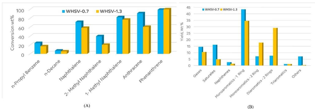
**Figure 5** Effect of WHSV on model feed conversion (Figure 5A) and (Figure 5B) product distribution. Reaction conditions: catalyst: Pt/Al<sub>2</sub>O<sub>3</sub> and Y zeolite (SAR-80) (1:1wt%), temp = 450°C, pressure = 60 bar, H<sub>2</sub>/HC = 10.
