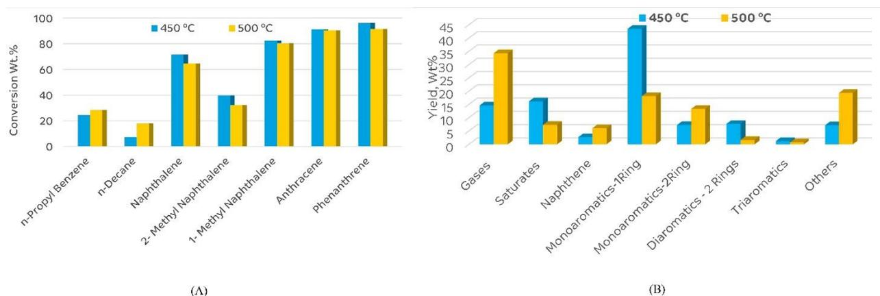
**Figure 4** (A) Effect of temperature on components conversion and (B) product distribution.
