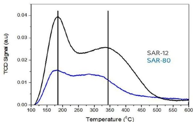
**Figure 3**  $\text{NH}_3$ -TPD results of Y zeolite with SAR-12 and SAR-80.
