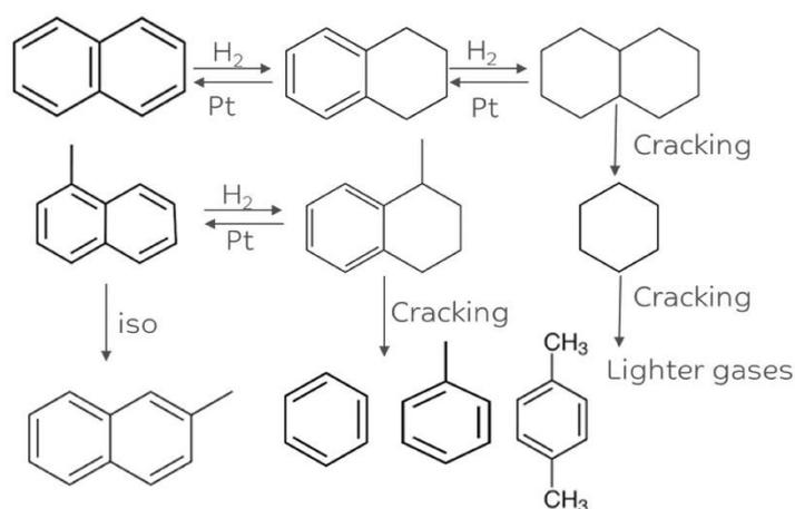
**Scheme 1** Plausible routes for different product distribution during hydrocracking reaction over bi-functional catalysts.
