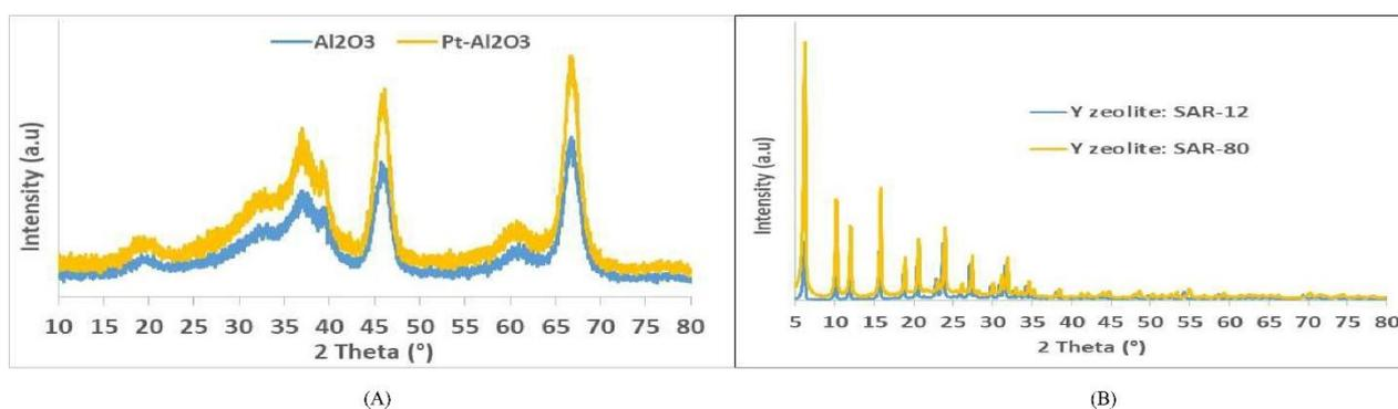
**Figure 1** XRD patterns of (A) Al<sub>2</sub>O<sub>3</sub>, Pt/Al<sub>2</sub>O<sub>3</sub>, (B) Y zeolite SAR-12 and 80 catalysts.
