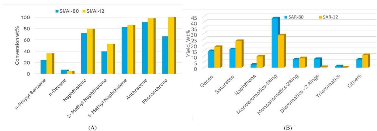
**Figure 7** Effect of Si/Al of Y zeolite on component conversion (Figure 7A) and product distribution (Figure 7B). Reaction conditions: catalyst-Pt/ $\text{Al}_2\text{O}_3$  and Y zeolite (1:1wt%), temperature-450°C, WHSV-0.7  $\text{h}^{-1}$ , pressure-60 bar,  $\text{H}_2/\text{HC}$ -10, TOS-22 h.
