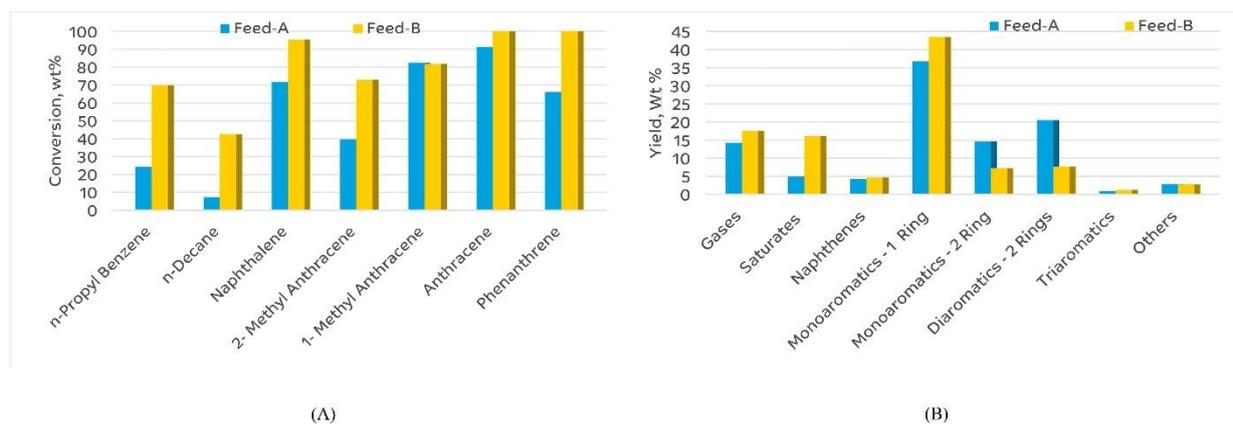
**Figure 8** Effect of paraffin concentration on components conversion (Figure 8A) and product distribution (Figure 8B). Reaction conditions: Feed A and B, Pt/Al<sub>2</sub>O<sub>3</sub> and Y zeolite (Si/Al-80) (1:1 wt%), temperature-450°C, WHSV-0.7 h<sup>-1</sup>, pressure-60 bar, H<sub>2</sub>/HC-10, TOS-22 h.
