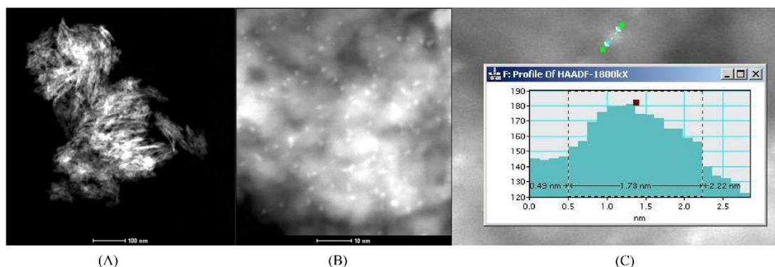
**Figure 2** HAADF-STEM (A, B) images and the Pt particle size distribution (C).
