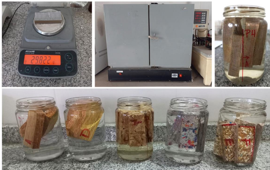
Figure 5 Water absorption test procedure.
