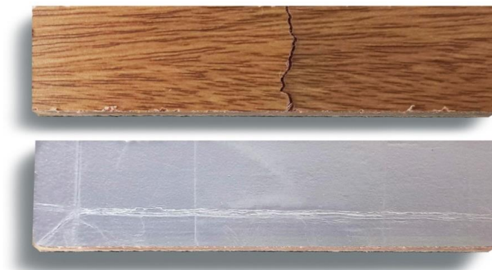
Figure 7 Particleboard and Tetrabrik specimens after being tested in flexion.
