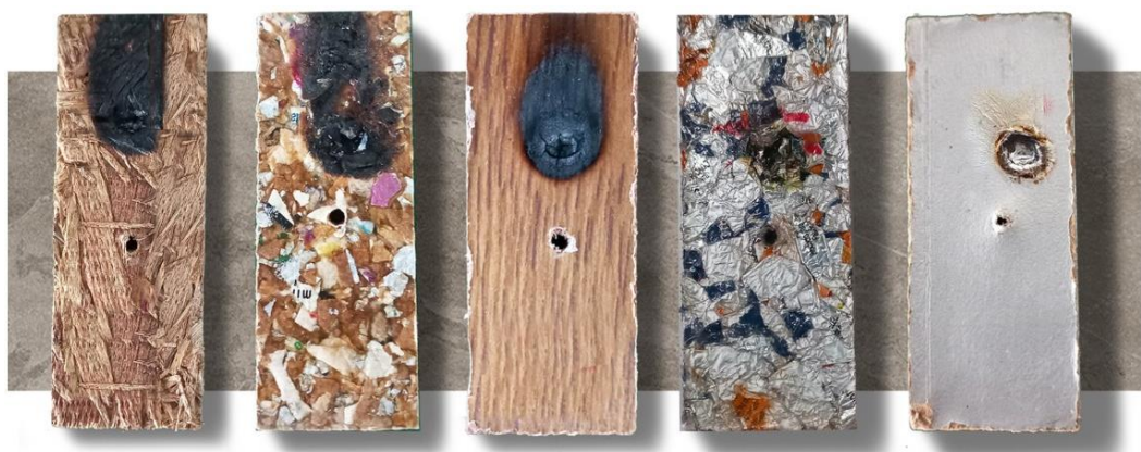
Figure 16 Flame mark on specimens: OSB, T-PLAK, Particleboard, Polyaluminum, and Tetrabrik.
