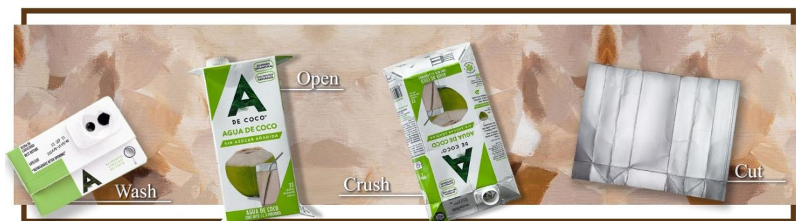
Figure 1 Preparation of TetraBrik packaging.
