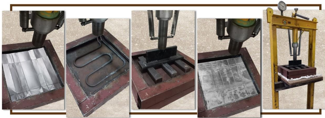
Figure 2 Manufacturing process of the boards.
