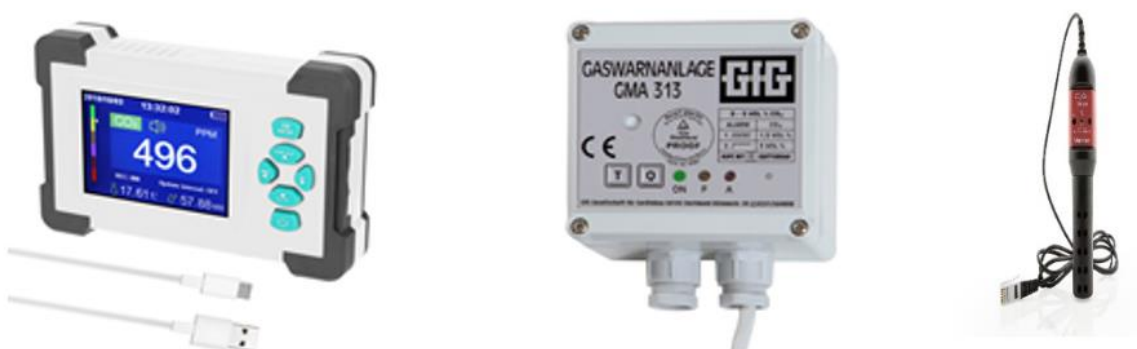
Figure 2 Carbon dioxide detector: domestic (left) [66] and professional (center) [67]. NDIR (right) [68].
