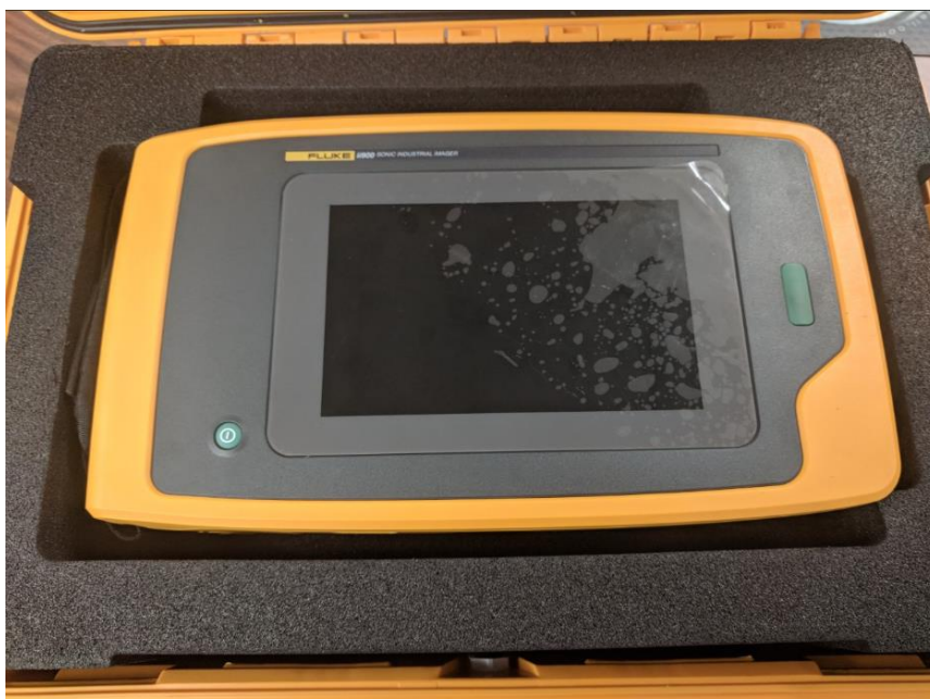
Figure 8 Fluke ii900 ultrasonic leak detector.
