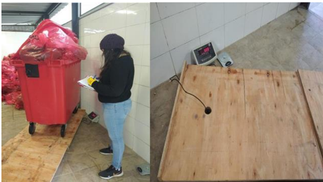
Figure 4 Platform designed by DIA IMFIA, to be used in HCW weighing and characterization.
