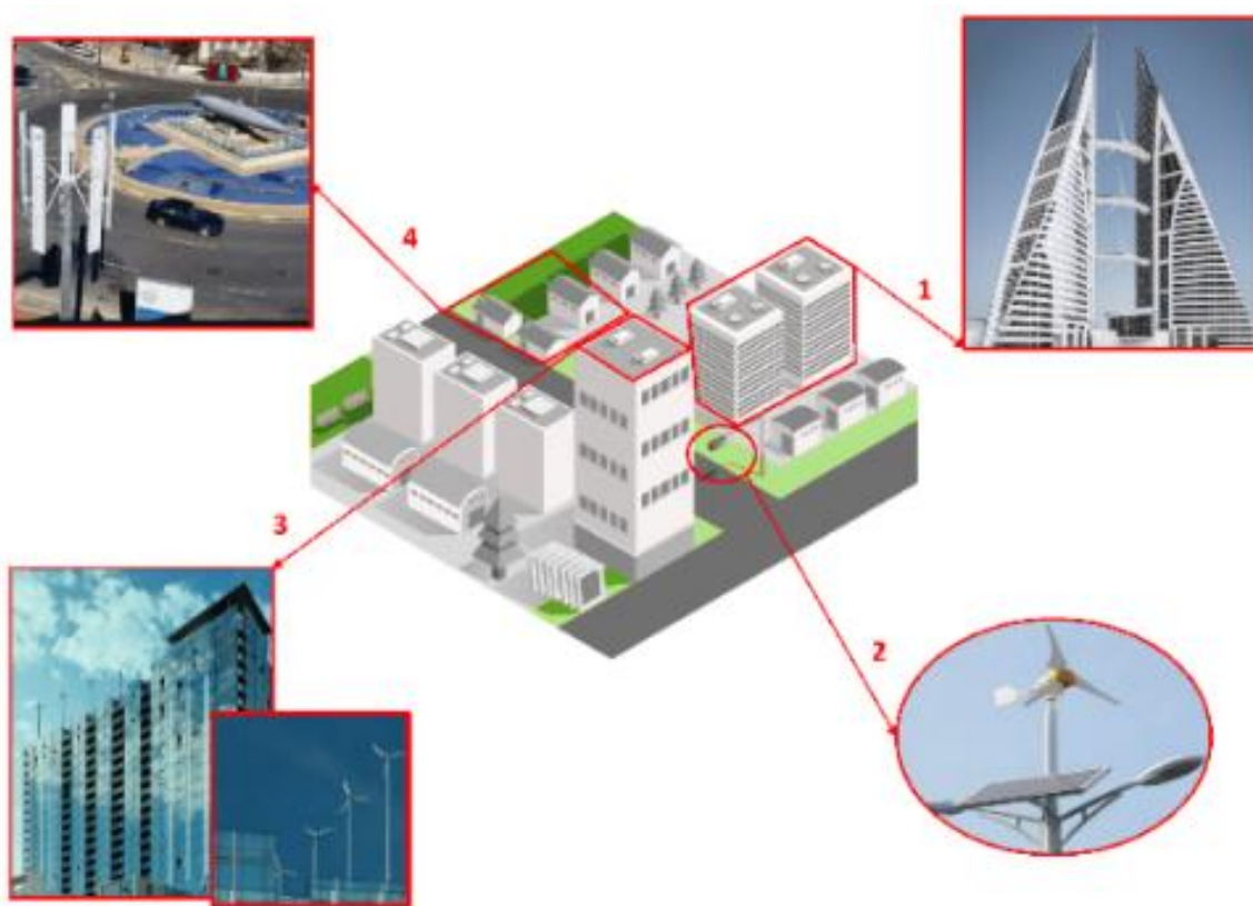
Figure 3 Types of urban wind energy collection systems: (1) Integrated; (2) Freestanding; (3) On the roofs of buildings; (4) Near buildings [32], permission for use authorized by Multidisciplinary Digital Publishing Institute, MDPI.
