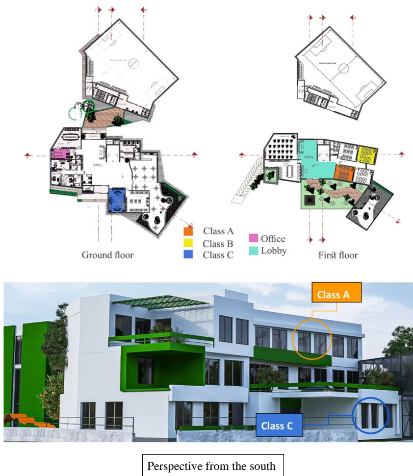
Figure 2 Ground Floor plan and perspective of the selected spaces for daylighting analysis.
